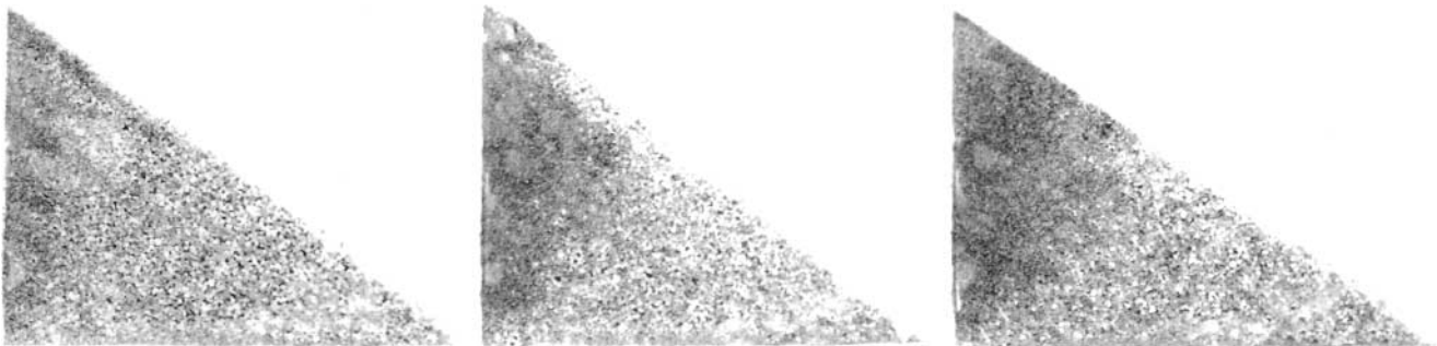
Fig. 5. Binary mixtures of quartz sand with (left to right) 60, 40, and 20% small grains. The small grains are colored black and tend to accumulate under the apex of the pile.
